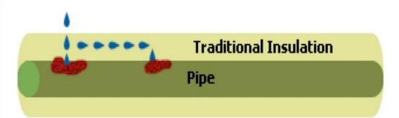
Rockwool, fiberglass, or other traditional types of insulation promote corrosion, and also act as a carrier and spread the corrosion to other areas of the pipeline
